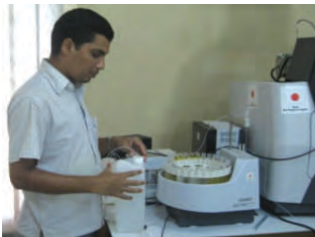
Photo: Measuring arsenic by AAS
