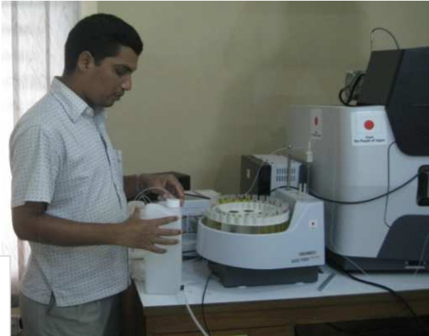
Photo 4: Measuring arsenic by AAS
